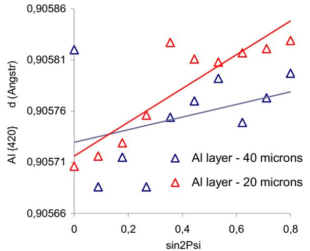
Figure 2. Effect of Al layer thickness on Residual stresses (Information Depth - 20 $\mu\text{m}$ )
