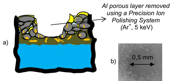
Figure 3. Removal of Al porous layer
