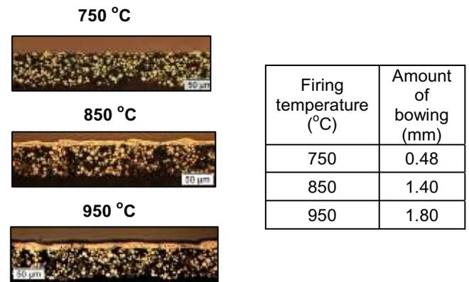
Figure 5. a) Effect of maximum firing temperature on microstructure of Al back contact layers, showing different thicknesses of the eutectic layer b) Resulting amount of bowing.
