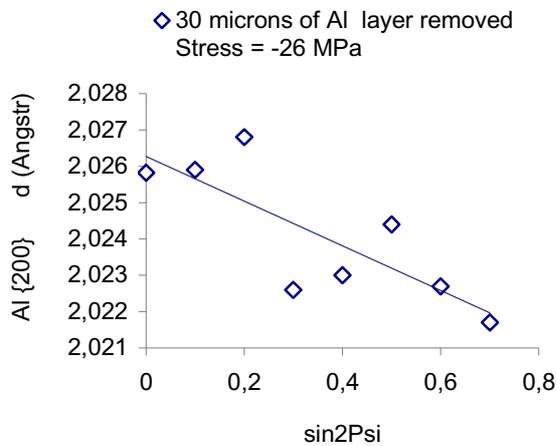
Figure 4. XRD stress result for the eutectic layer (sample with removed Al layer)
