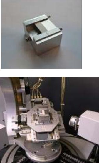
Figure 1. In-situ bending clamping device for XRD
