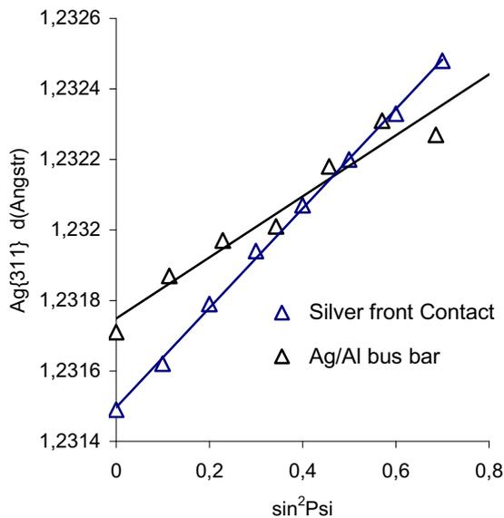
Figure 8. Residual Stresses in Silver front contact and Silver Bus bar (Penetration Depth ~ 2 µm)
