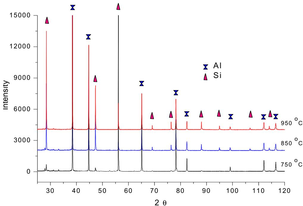
Figure 6. XRD pattern of Aluminum layer fired at 750, 850 and 950 °C
